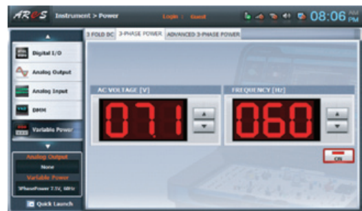
3-Phase Variable AC Power supply
