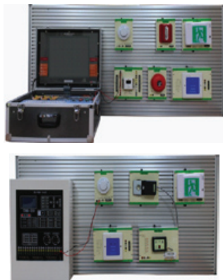
Fire Fighting Electrical Wiring Device Application
