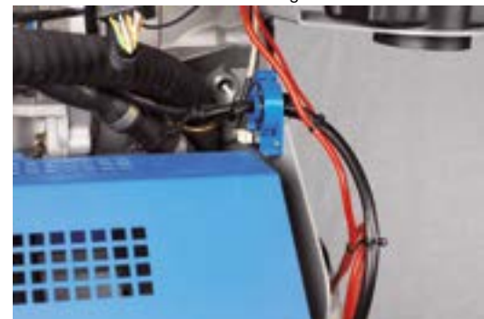
Sensor for measuring current.
