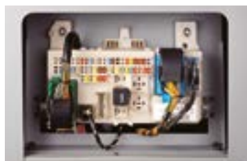
Fuse and relay box (GEM module).
