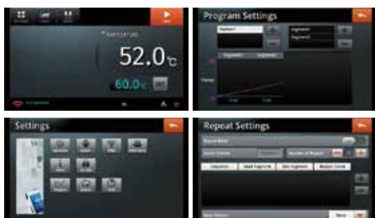
4” Full Touch Screen TFT LCD (Smart-Lab™ Controller)
