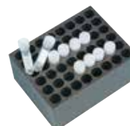
(4) "BLT248" For φ 12mm Tube. (φ 12×h35mm)×48 holes, Round Bottom Holes
