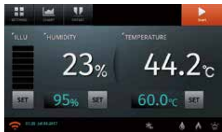
7" Full Touch Screen TFT LCD (Smart-Lab™ Controller)
