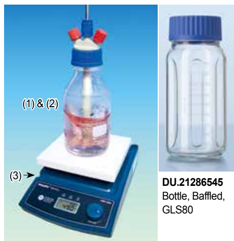
(2) GLS 80 Stirred Reactor-set, w/4-port
