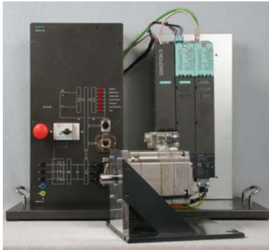
SINAMICS S120 1,5 kW, power feeding in network; frequency converter with SIMOTION D module
