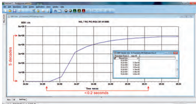
HPR-20 transient MS data - > 5 decades response in < 0.2 s
