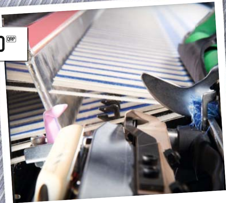
Optimized shed geometry
