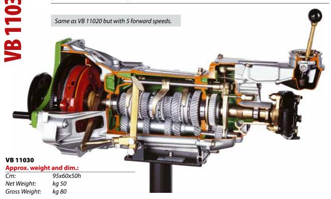
These cutaway models are carefully <u>sectioned</u> for training purposes, professionally <u>painted</u> with different colours to better differentiate the various parts.
