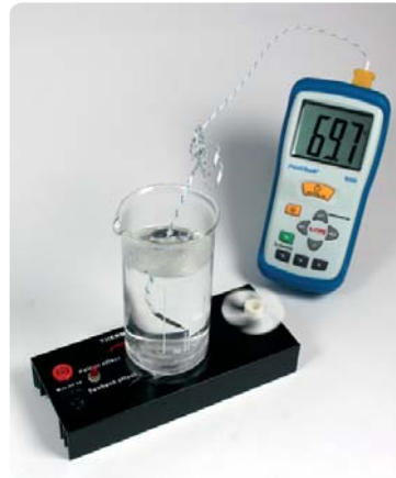
Stand set-up: „Conversion of thermal energy into electric energy“
