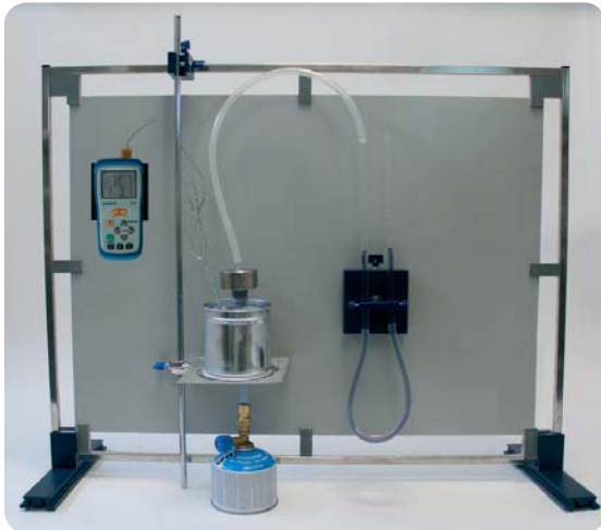
Magnetic board set-up: "Volume change at a constant pressure"
