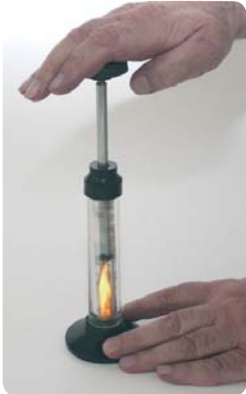
"Heating of air when compressed"
