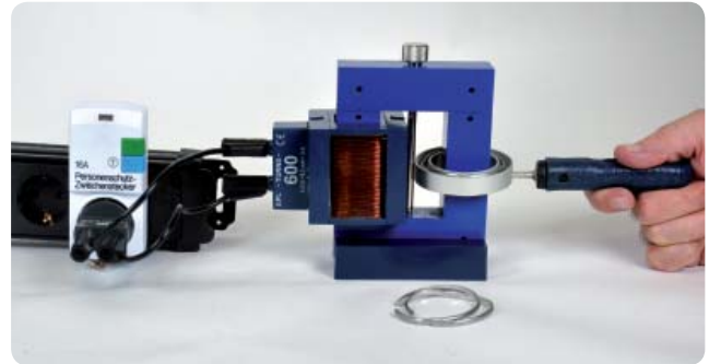
Model experiment: "High-current melting with the melting ring"
