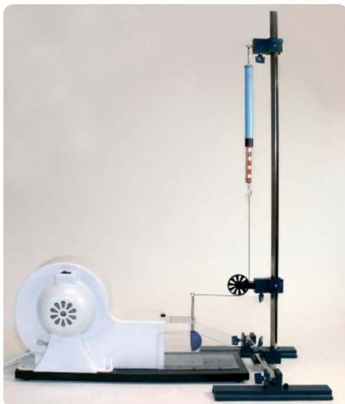
"Measuring the drag coefficient of a hemisphere"
