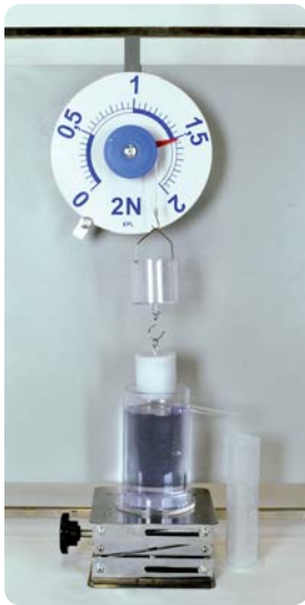
Magnetic board set-up: "Archimedes' principle"
