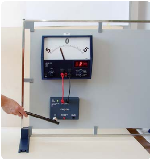
"Displaying the negative load of a ground ebonite rod"
