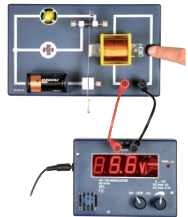
"Relay – Normally open and normally closed contact"
