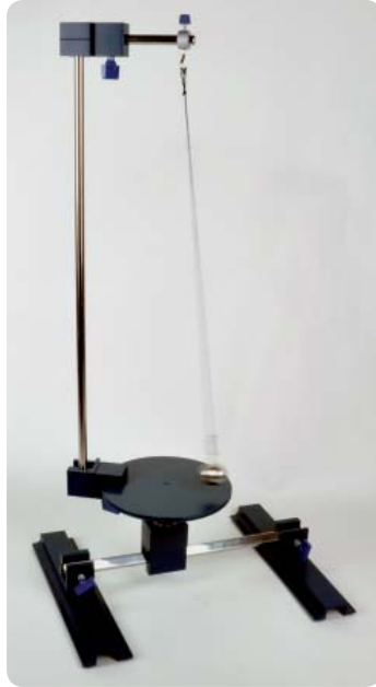
Stand set-up: "Foucault pendulum" with: Bearing unit, long, and belt pulley
