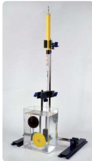
"Measuring the buoyancy of a polystyrene ball"
