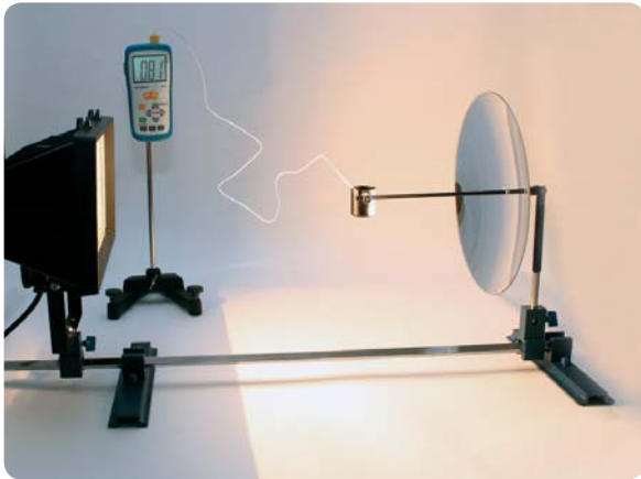
Stand set-up: „Reflection of thermal radiation“
