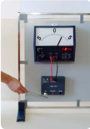
Magnetic board set-up: "Displaying the positive charging of an acrylic glass rod using an electrometer amplifier"
