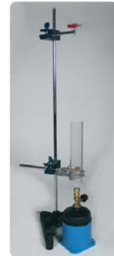
Stand set-up: „Thermal convection“
