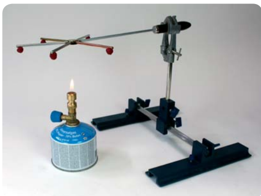
Stand set-up: "Thermal conduction in different metal bars"
