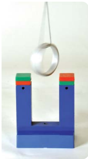
Experiment: „Braking effect on a rotating aluminium ring in the magnetic field of a U-magnet“
