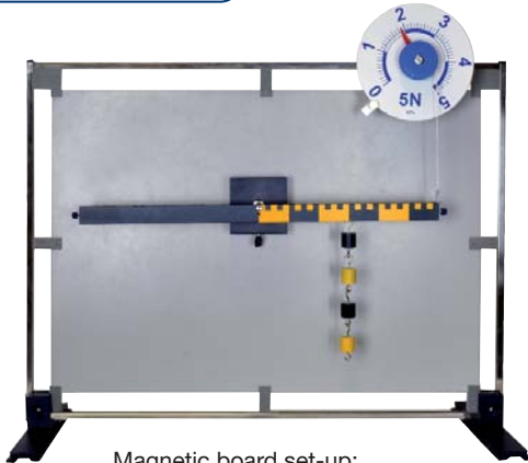
Magnetic board set-up: "Single-sided lever"
