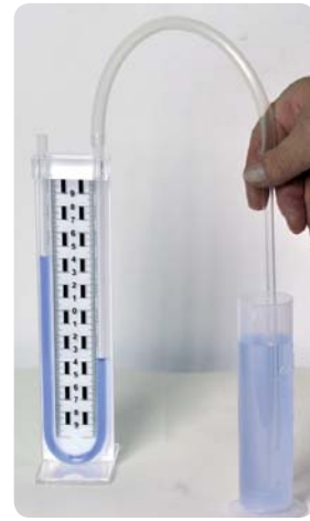
„Measuring the hydrostatic pressure“ with submersible probes
