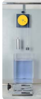
Magnetic board set-up: "Buoyancy of objects with different densities"
