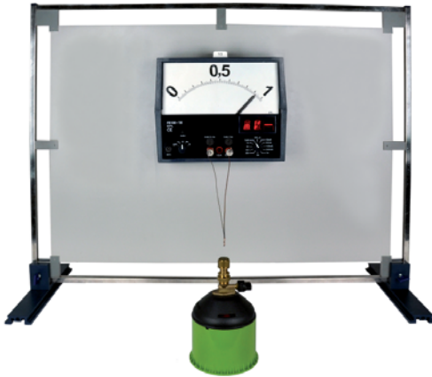
Magnetic board set-up: „Converting thermal energy to electrical energy“
