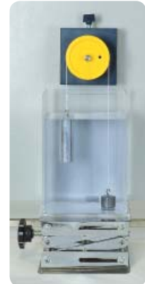
Magnetic board set-up: "Buoyancy of objects with different densities"
