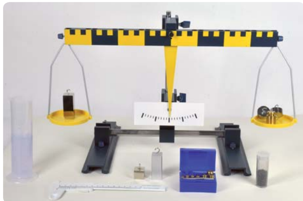
„Determination of the density of solids with built-up scales“
