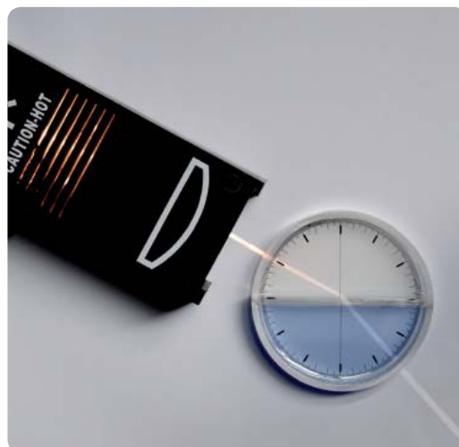
"Refraction during transition from air into water" (use of the circular cell)
