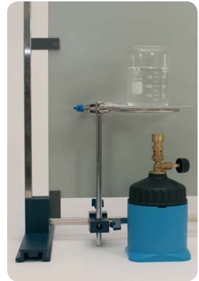
Mounting the heat protection net on the square frame of the assembly plate
