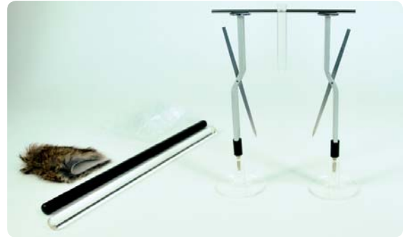
„Separation of charge by electrostatic induction“
