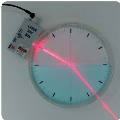
„Refraction with laser ray box“
