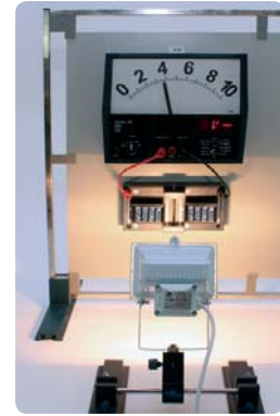
Magnetic board set-up: „Series connection of photovoltaic cells – Measuring the voltage“
