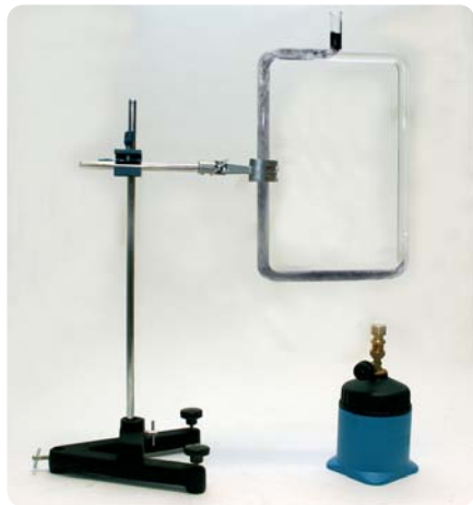
Stand set-up: "Thermal convection in water"
