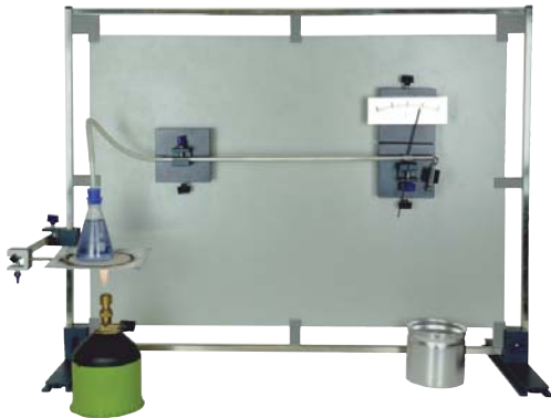
Magnetic board set-up: „Linear expansion of metal tubes“
