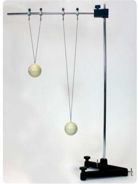
Stand set-up: „Pendulum with different lengths“
