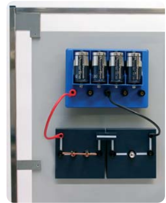
Magnetic board set-up: "Conductors and non-conductors"
