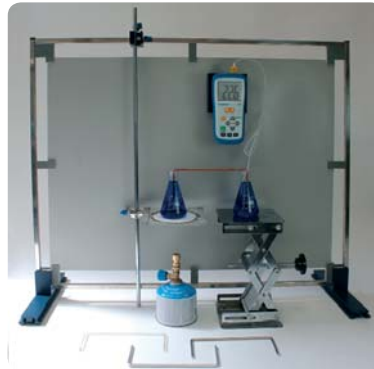
Magnetic board set-up: „Thermal conduction in solid objects“
