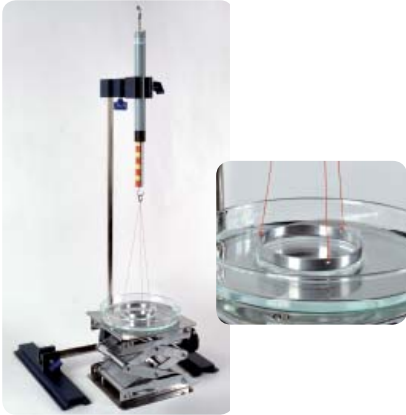
"Measuring the surface tension of water" with the 0.1 N dynamometer
