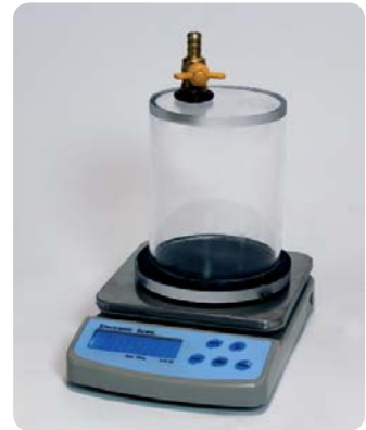
"Weight of displaced air 1 litre: 1.3 grams"
