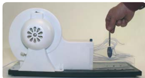
"Wind tunnel: Vortex formation on a circular plate"
