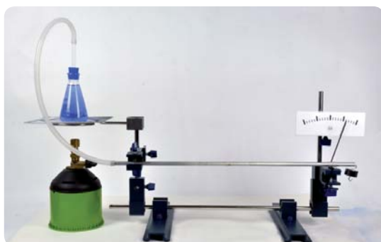
"Linear expansion of solids"
