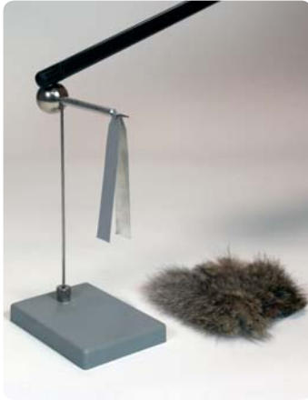
Stand set-up: "Leaf electroscope"
