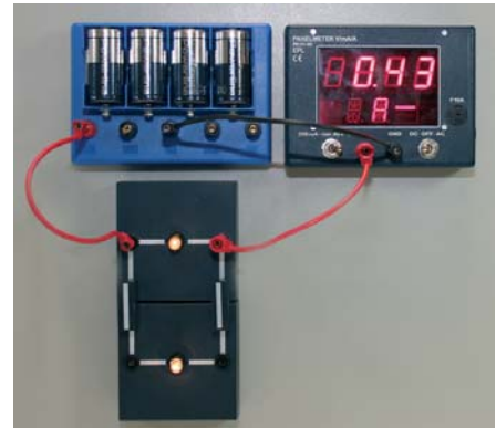
"Parallel connection of light bulbs"
