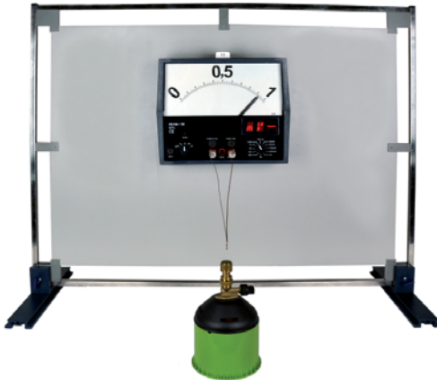
Magnetic board set-up: "Conversion of thermal energy into electric energy"
