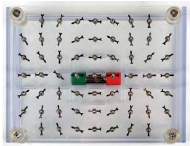
"Field pattern of a bar magnet" (Suitable for overhead projection)
