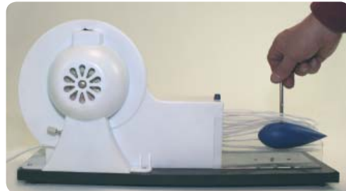
"Wind tunnel: Irrotational streamlined body"
