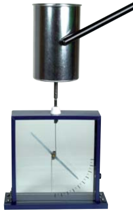
"Charge distribution to a metallic hollow object"
