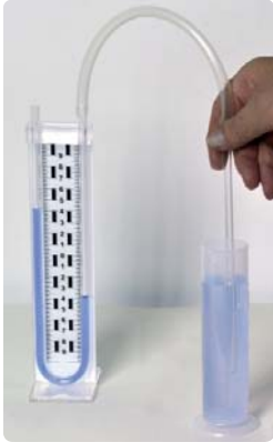
„Measuring hydrostatic pressure“
