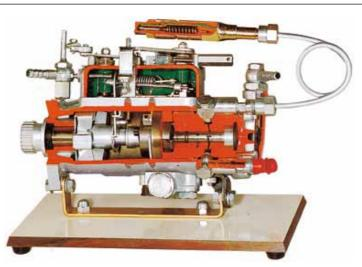
Careful section of a CAV rotary pump for training purposes, showing all its operating parts.
