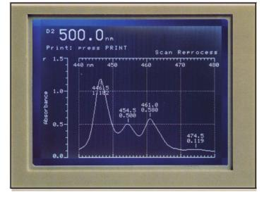
A combined cell and wavelength program may be run for up to 8 cells and 10 wavelengths.
