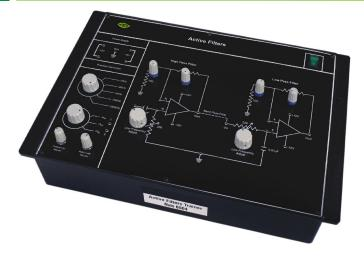
**Nvis 6504 Experimentation with Active Filters** is a remarkable and frequently used laboratory equipment which is designed to explain basic fundamentals of filter design and their working. Electronic filters are electronic circuits which perform signal processing functions, specifically intended to remove unwanted signal components and/or enhance wanted ones.
