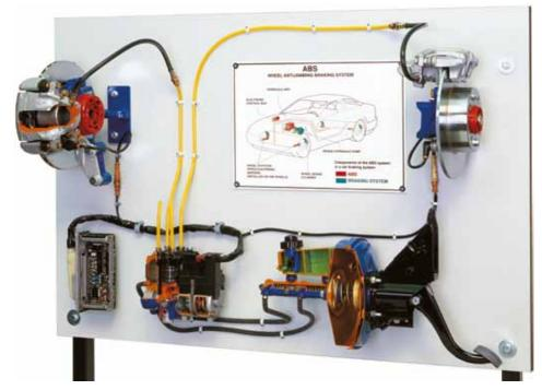
Educational model of a modern ABS braking system for motorcars. All the brake parts are provided as detailed cutaway models, connected together to enable easy understanding of the brake assembly operation.
