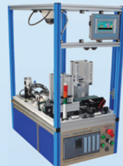
Distribution Station (CPE-FAS30A)
