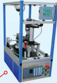
2nd Test & Sorting Station (CPE-FAS30E)
