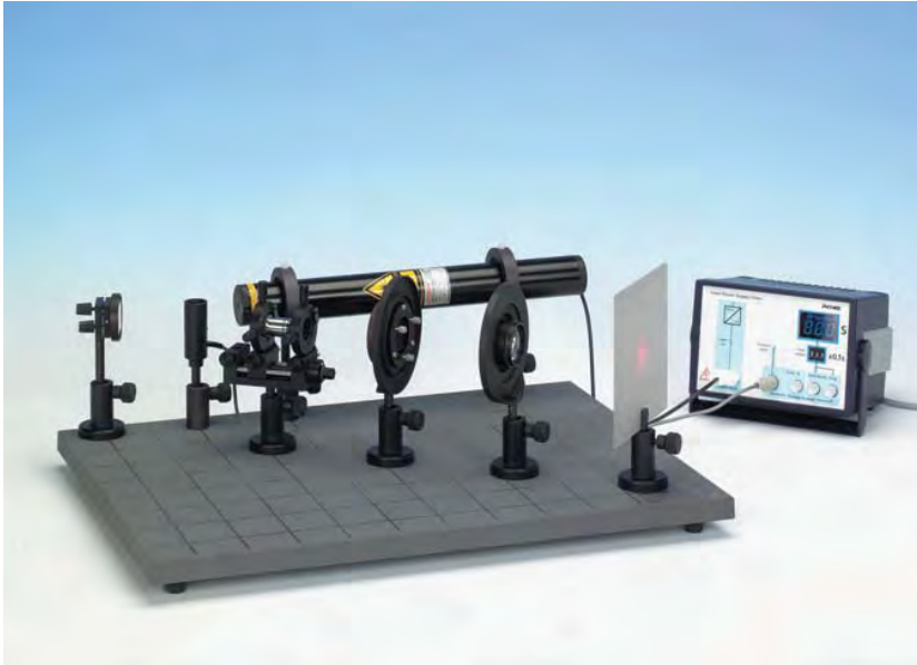
Generation of Newton's rings.
