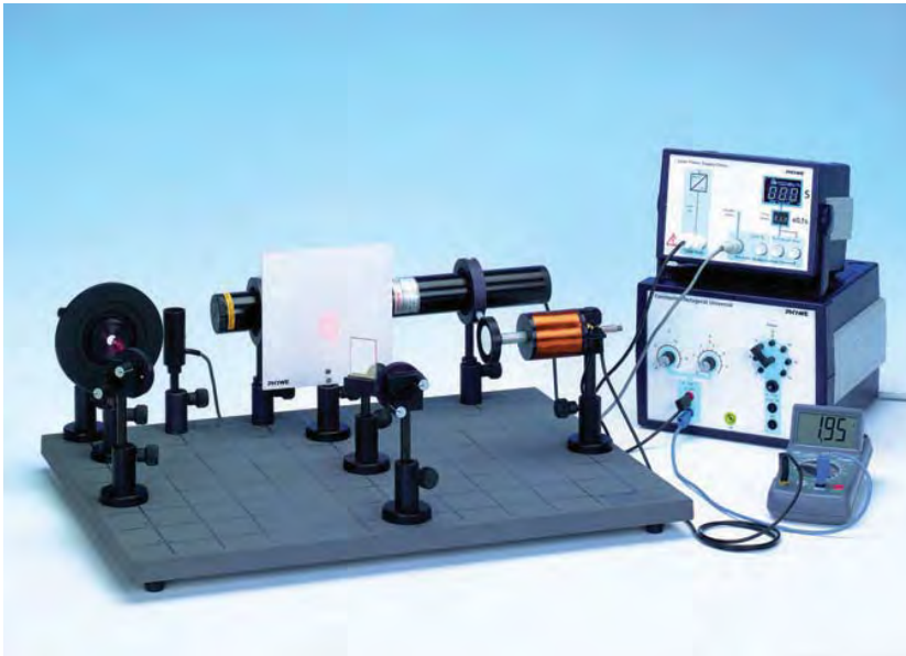
Formation of circular interference fringes.
