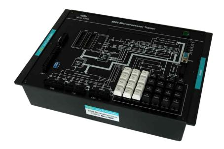
Nvis 5586 is a product based on INTEL 8086 Microprocessor for purpose of training and development of Microprocessor based systems. It provides a simple platform for the students to learn the concepts of 8086 architecture, its assembly language programming, interfacing and working of different peripherals used in 8086 based system. The training board is very user friendly and self contained allowing students to carry out practical work and gain knowledge about Microprocessor based systems.
