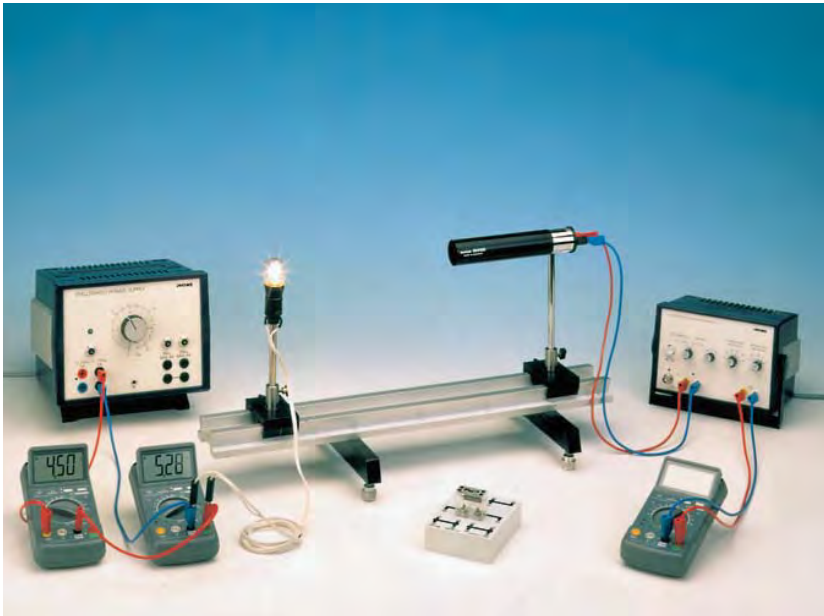
Thermoelectric e. m. f. of thermopile as a function of the filament's absolute temperature.
