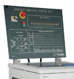
Washing Machine Training Set has been designed to operate and observe the washing machine system structure and theory as well as to know about circuit elements and to serve for applied training.
