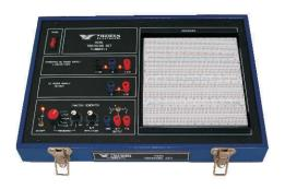
Advanced Project Application Board is designed to do basic and advanced electronics applications. There are Power Supplies, function generator and portable breadboard on the set. The power supplies on the set can operate as symmetrical or TTL.
