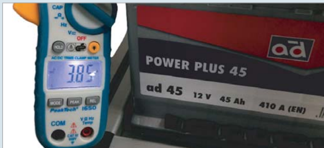
Charging current with consumer connected approximately 230 W at around 2000 rpm
