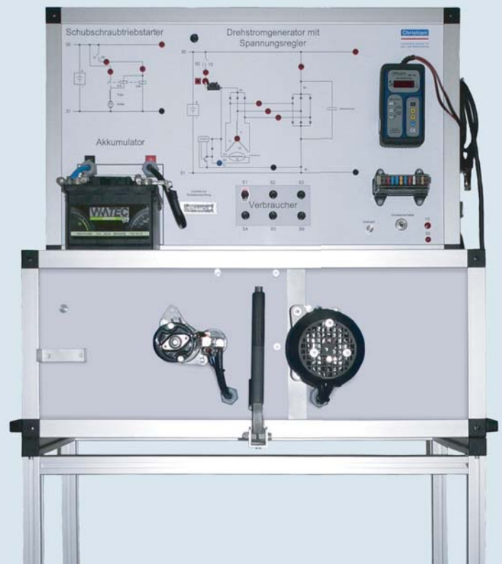
Charging current with consumer connected approximately 230 W at around 2000 rpm
