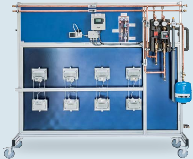
S3 solar collector with solar simulation
