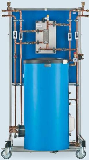
S4 hydraulic switch, plate heat exchanger and buffer storage
