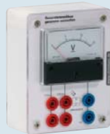
Generator connection (voltmeter)
