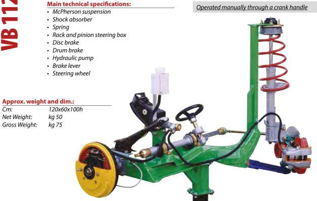
These cutaway models are carefully sectioned for training purposes, professionally painted with different colours to better differentiate the various parts.
