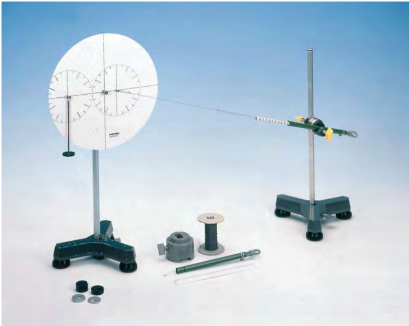
Moment as a function of the distance between the origin of the coordinates and the point of action of the force.
